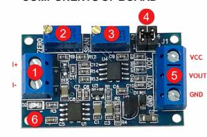
No.1 Terminal provides Input Current (0-20mA, 4-20mA); in this case, I+ is Input Current and I- is Output Current.
