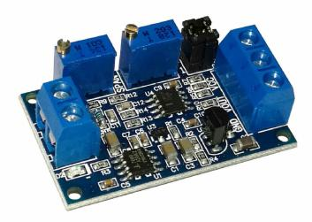
This completed board set is an imported product from aboard that can convert the Current 4-20mA into 0-5V; so, it can to connect to Circuit A TO D of Board Microcontrollers conveniently, for example, it connects from SENSOR devices that have OUTPUT in the format of 4-20mA.
